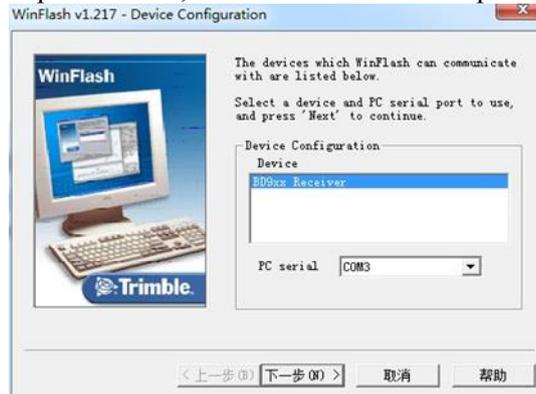
Step 5: After installation is completed, run “winflash” software. Following prompt on the screen, select serial port number of C18, and press “Next” button.
